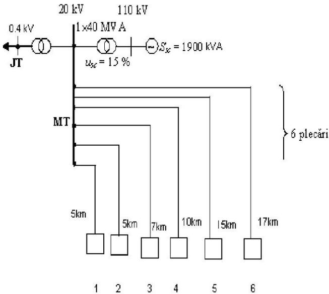
**Fig 4. The distribution network with six lines and one task per each line.**
