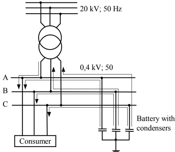
Fig. 1 – The circulation of the reactive power on the three phases of the analyzed consumer.
